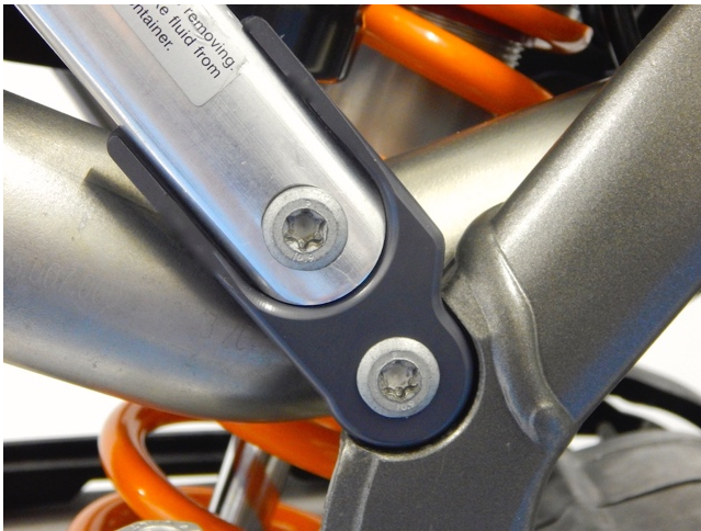
Both Lower brackets are completely identical. Other side will face down.
